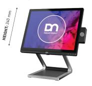
Height: 240 mm Width: 339 mm Depth: 38 mm Weight: 1.1 kg (without stand) 4.2 kg (with stand)
